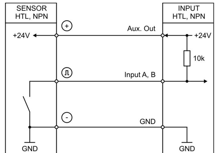
Unconnected PNP inputs are always "LOW" and unconnected NPN inputs are always "HIGH". All inputs are designed to receive impulses from electrical impulse sources.
