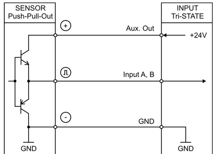
Unconnected PNP inputs are always "LOW" and unconnected NPN inputs are always "HIGH".
