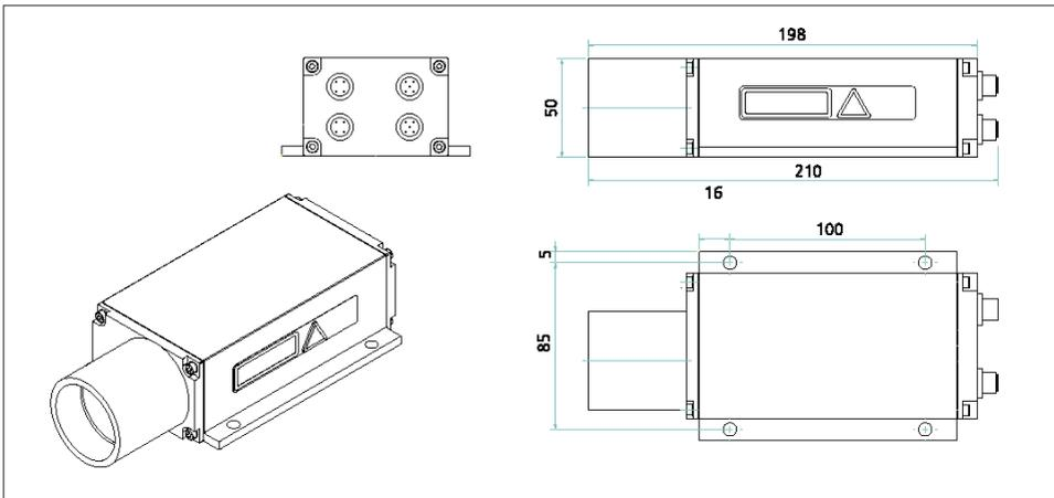
**Figure 3 : Mounting drawing**
